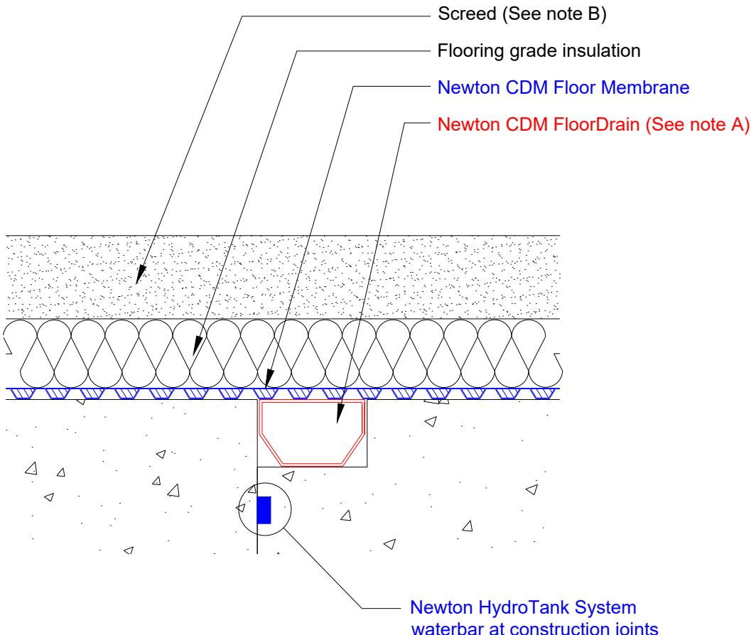
This detail shows protection to construction joints within the slab or raft with a line of Newton CDM FloorDrain. Use in conjunction with Newton drawings starting CDM-SW or CDM-RW where the Newton CDM BaseDrain is set within a recess to the slab or raft. If the Newton CDM BaseDrain is laid above the slab as with drawings starting CDM-SA or CDM-RA, detail CDM-D01 should be used.
