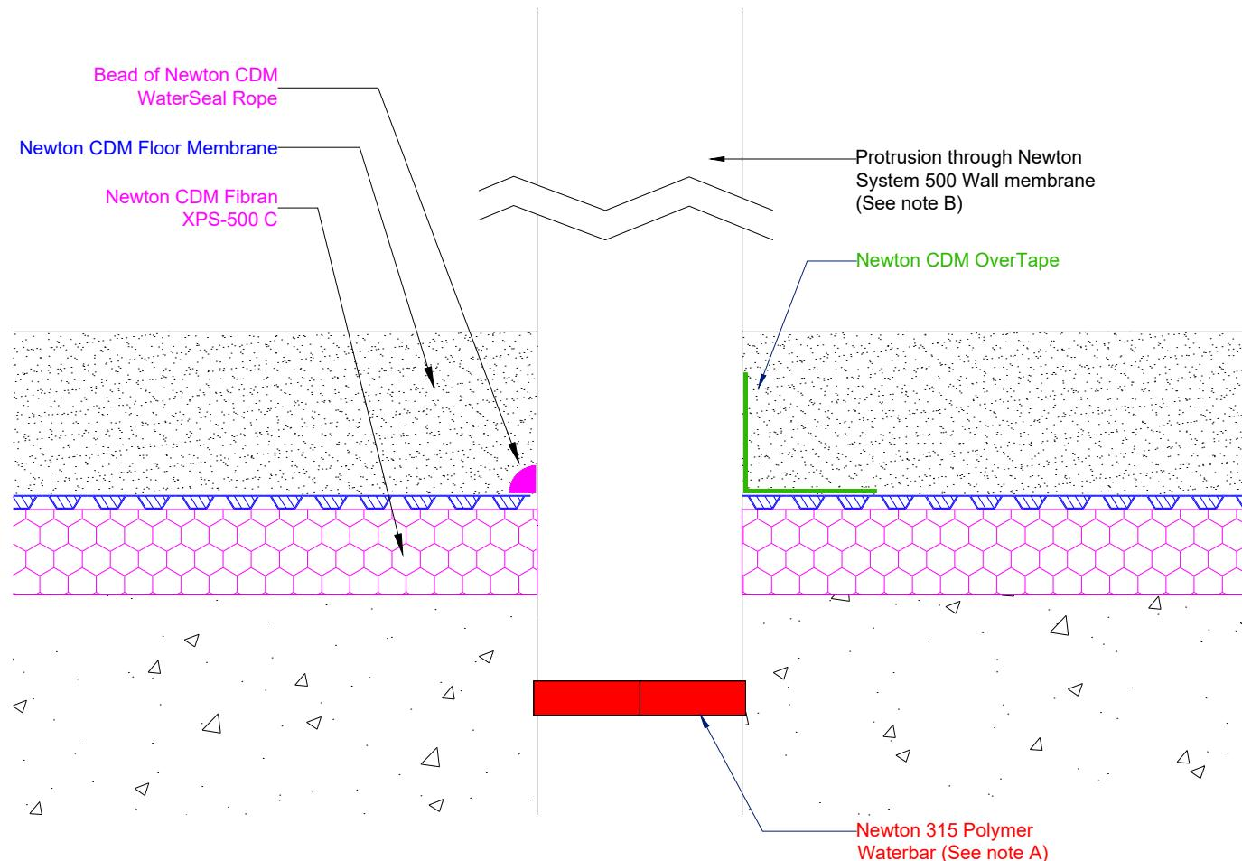
This detail shows a protrusion, such as a pipe or steel, through the Newton System 500 Floor membrane, showing sealing with Newton WaterSeal Rope or Newton CDM OverTape as options.,
