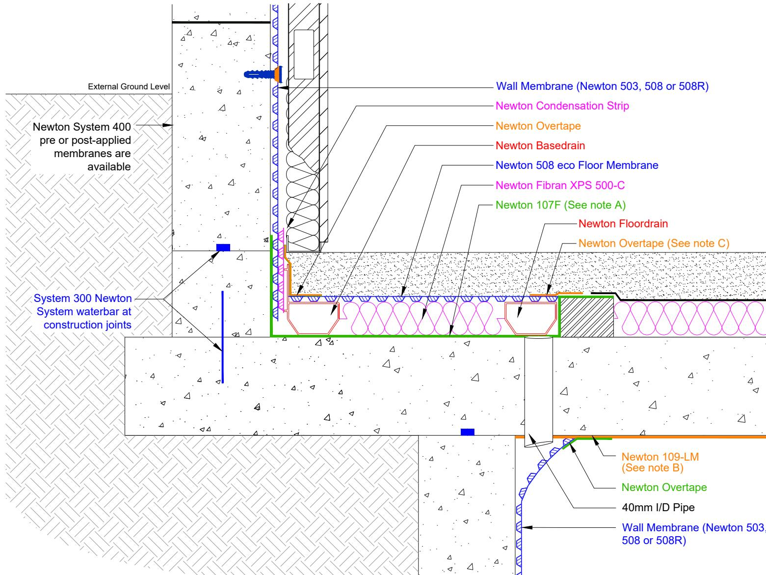
This detail shows a method of draining water through an abutting intermediate slab so that it can be received by the the Newton waterproofing system at the lowest level of the basement.
