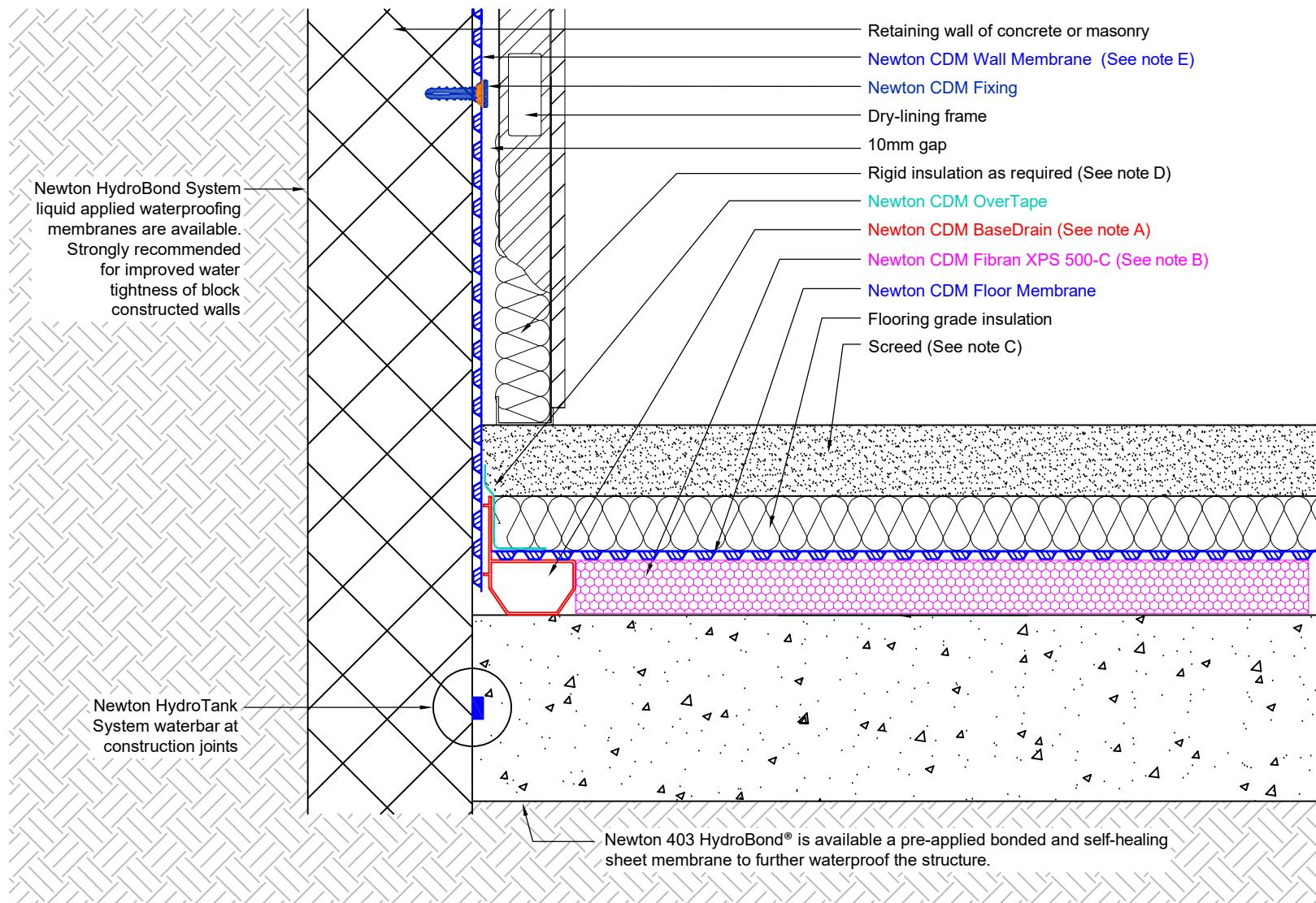
This detail assumes that the slab is in good condition - constructed to BS EN 1992 (Eurocode 2), and that the structure as a whole is of sufficient mass and quality to resist heads of water pressure as required by BS8102.
