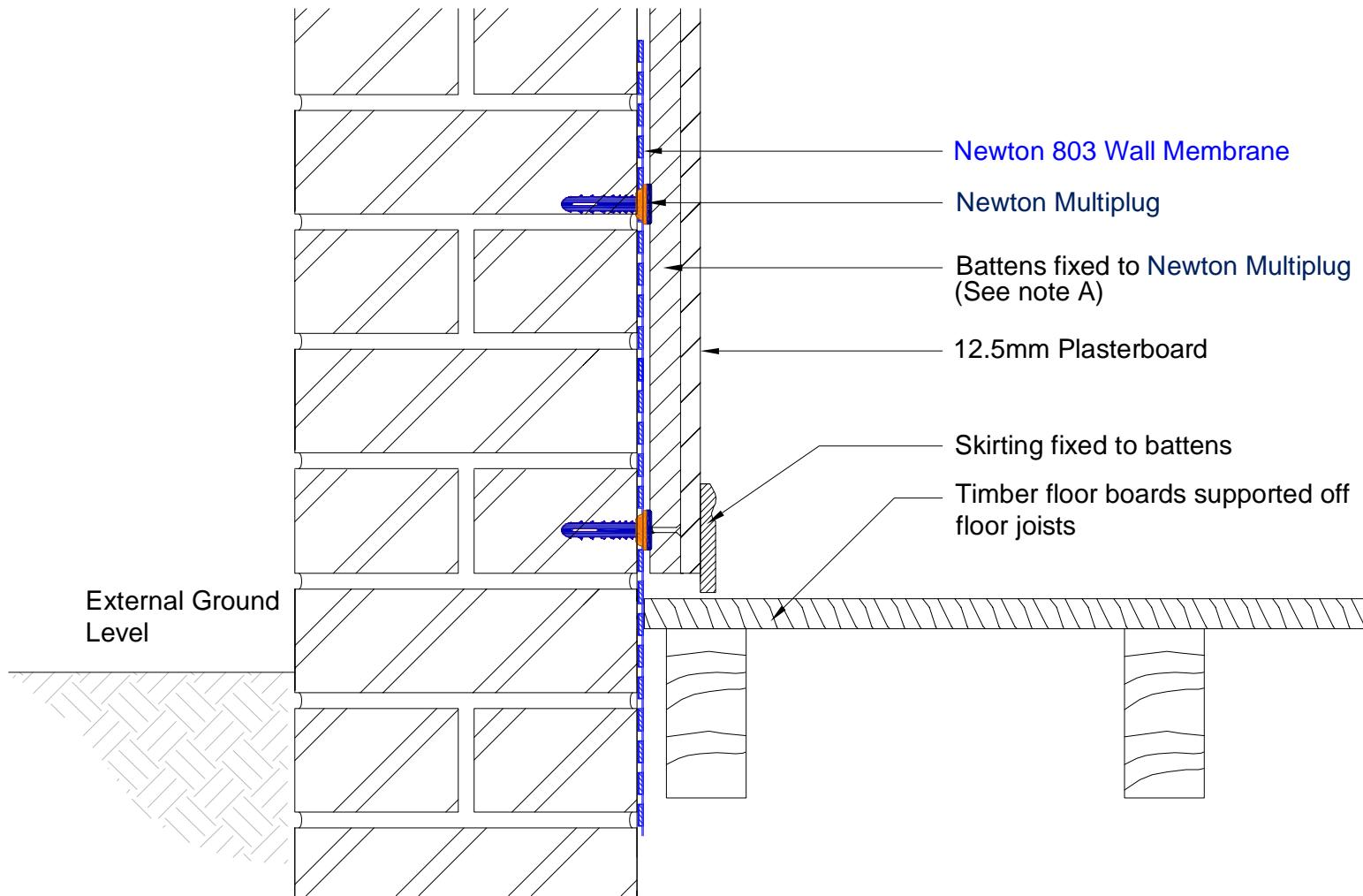
NOTE: This is a Newton damp proofing detail and copyright remains with John Newton & Co. Ltd. (trading as Newton Waterproofing Systems). Any specification/advice provided is only valid if used with products supplied by John Newton & Co. Ltd. For the design of the structure, please use a professional designer. Please refer to product data sheets before installation of our products. Newton Waterproofing Systems reserve the right to update drawings and product literature at any time.
