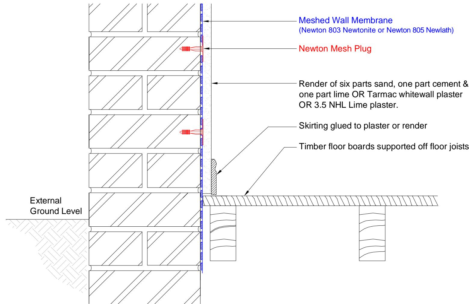
This drawing shows Newton 803 Newtonite or Newton 805 Newlath to the wall as a damp proofing solution.
