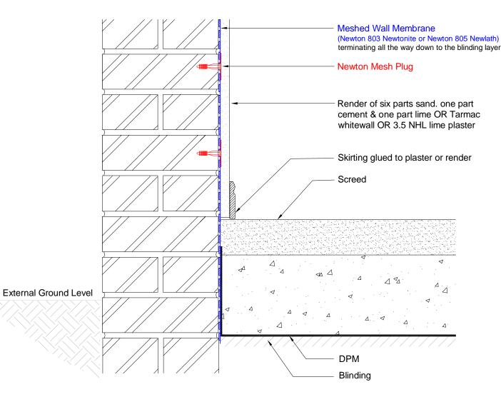
NOTE: This is a damp proofing detail. Please refer to product data sheets before installation of our products. Newton Waterproofing Systems reserves the right to update drawings.
