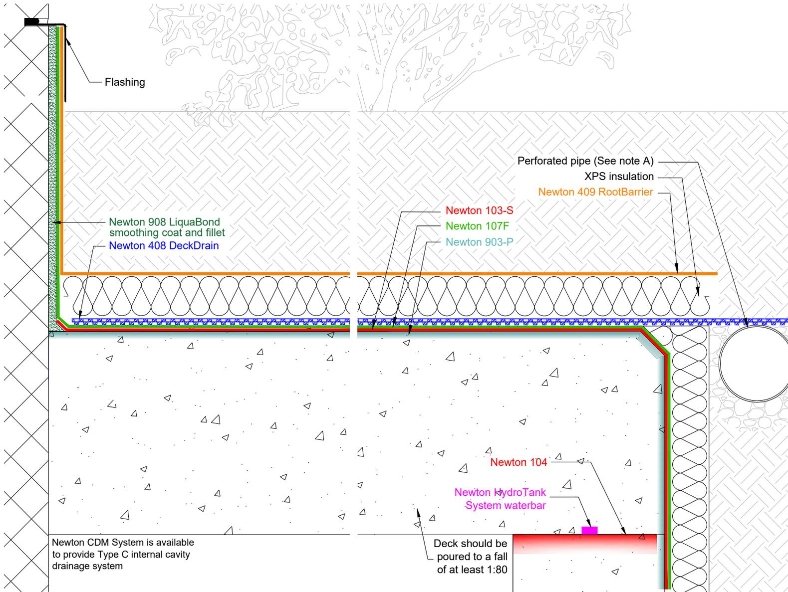
This drawing shows an intensive green roof specification where Newton 103-S and Newton 107F are providing the primary waterproofing to an Inverted Warm RC Deck.
