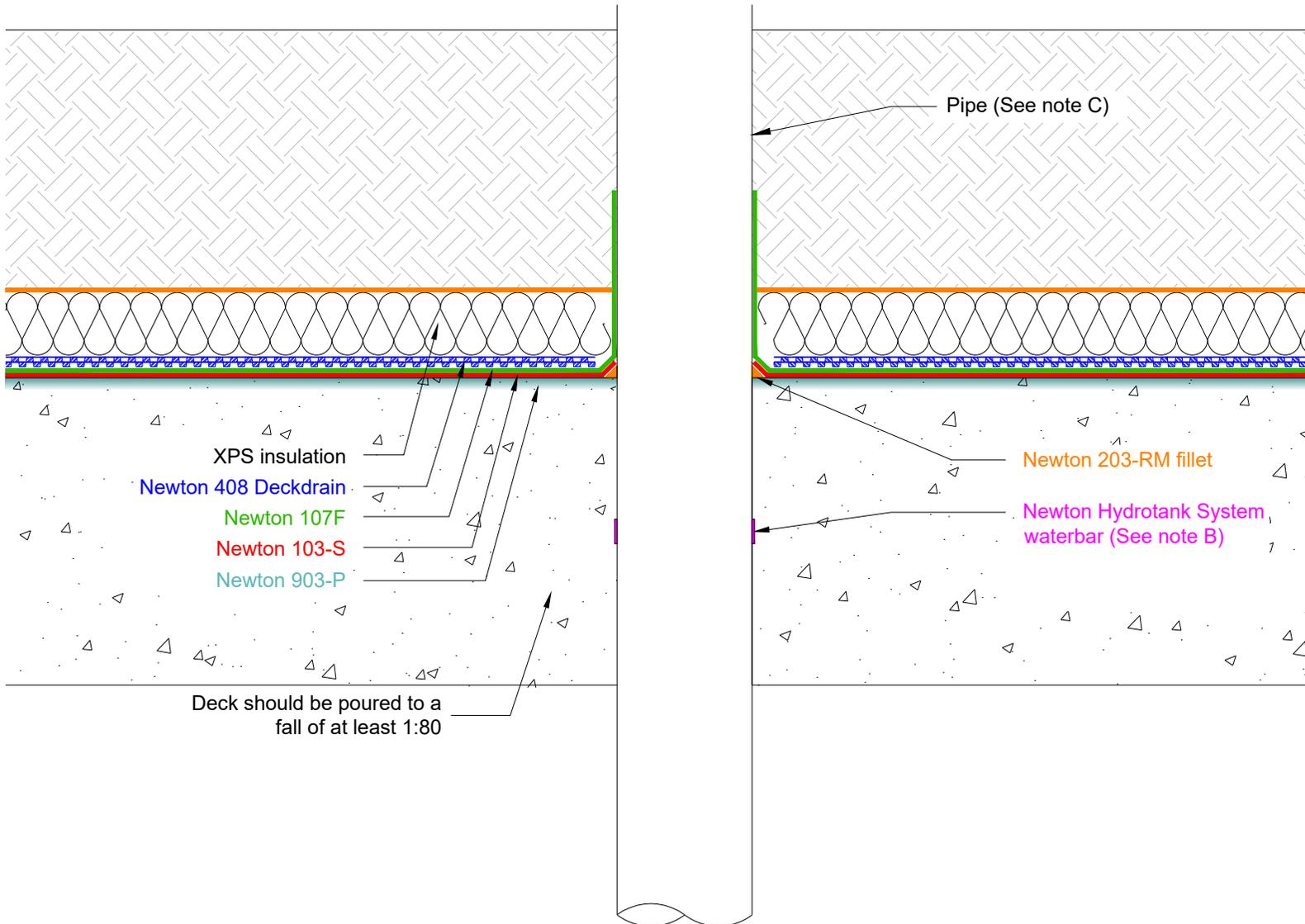
This drawing shows an intensive green roof specification where Newton 103-S and Newton 107F are providing the primary waterproofing to an Inverted Warm RC Deck.
