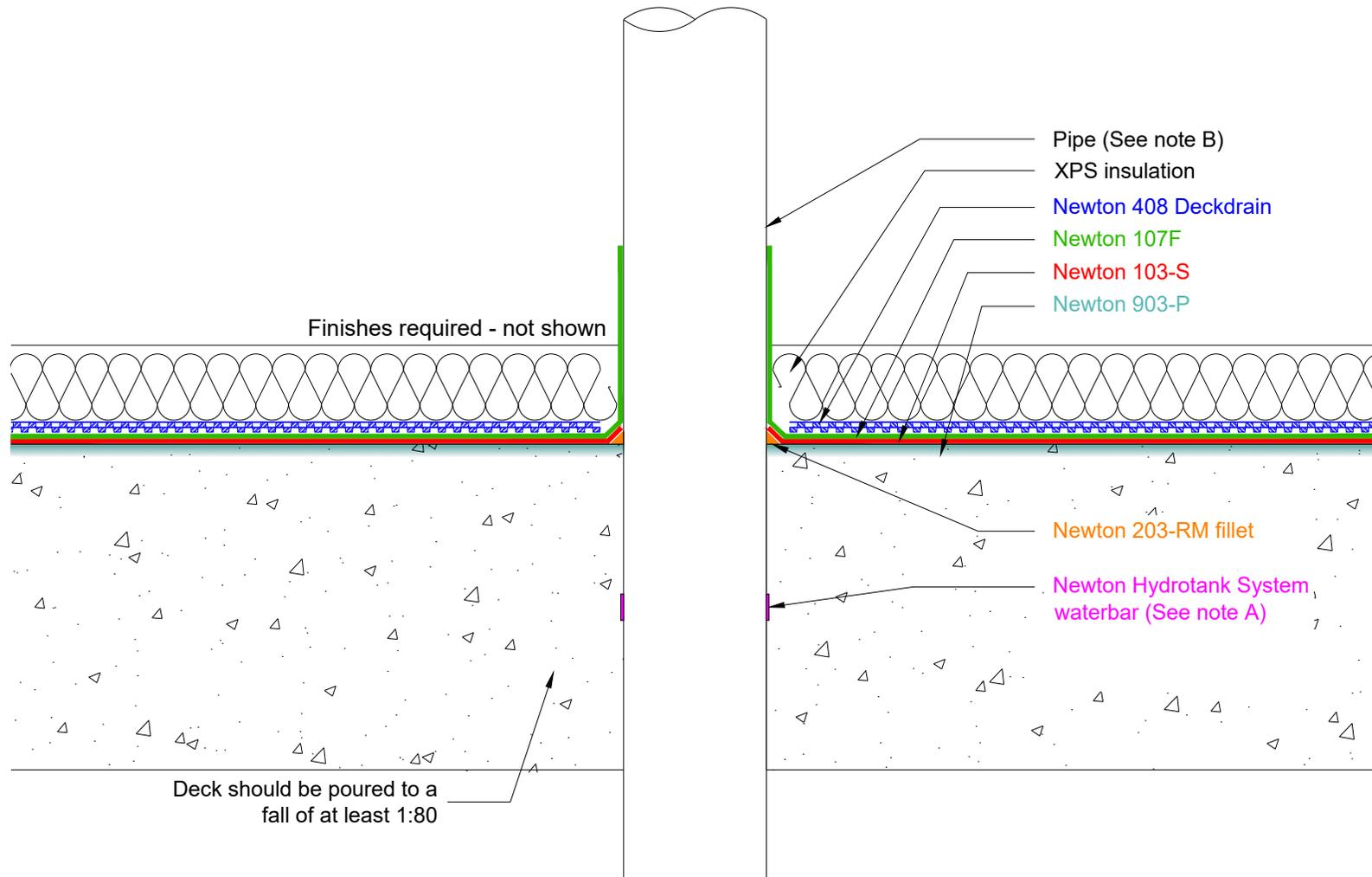
This drawing shows an extensive green roof specification where Newton 103-S and Newton 107F are providing the primary waterproofing to an Inverted Warm reinforced concrete deck.
