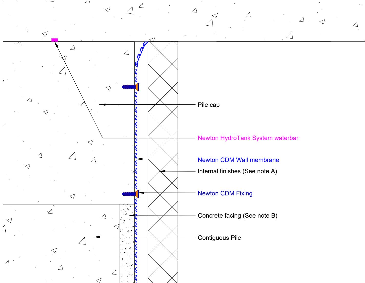
This detail shows the termination of Newton CDM System in front of Contiguous piles.
