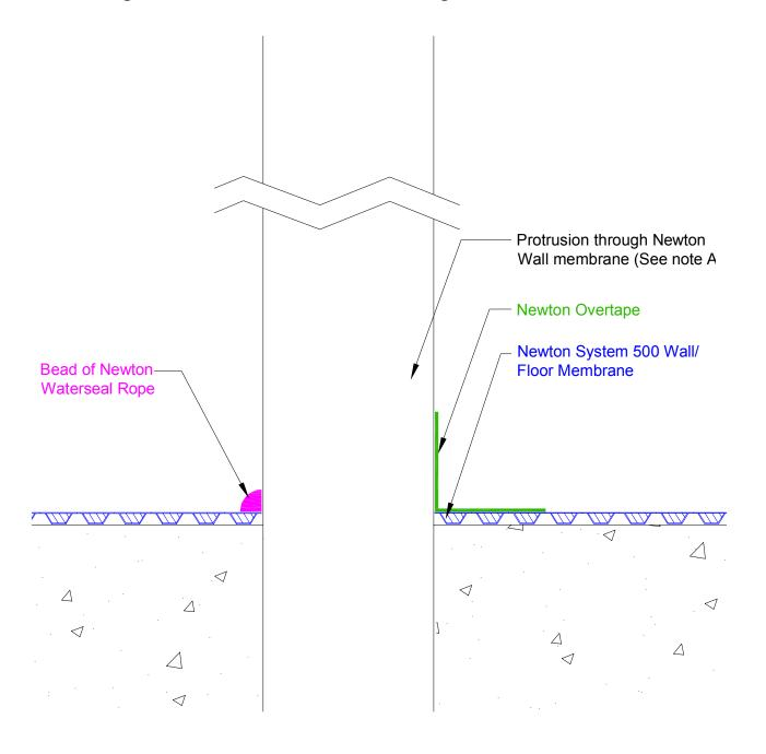
This detail shows a protrusion, such as a pipe or steel, through the Newton System 500 Wall/Floor membrane, showing sealing with Newton Waterseal Rope or Newton Overtape as options. This detail should be used in conjunction with Newton System 500 drawings prefixed RA or SA.
