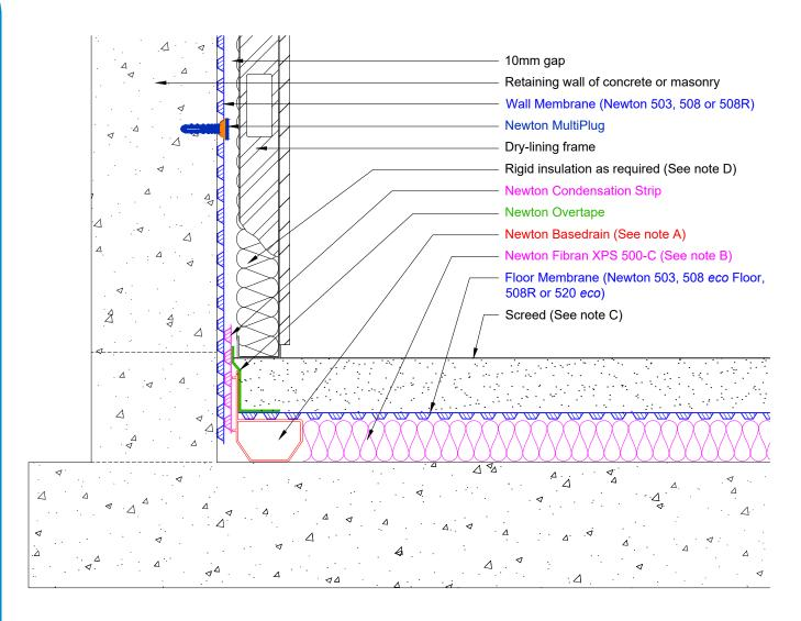
This detail assumes that the raft is in good condition - constructed to BS EN 1992 (Eurocode 2), and that the structure as a whole is of sufficient mass and quality to resist heads of water pressure as required by BS8102.
