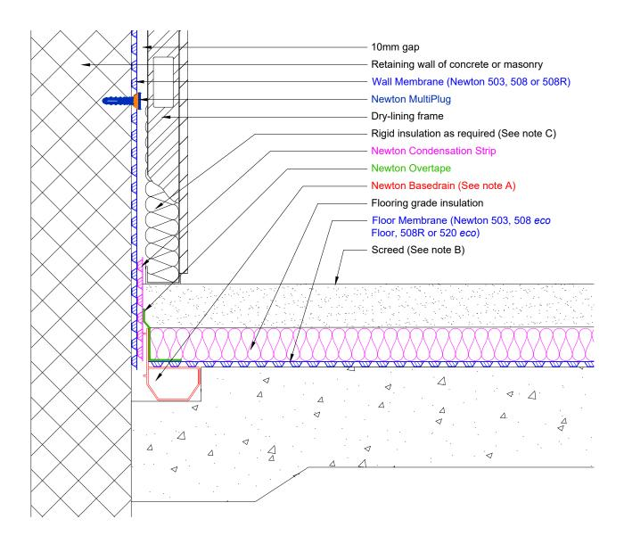
This detail assumes that the slab is in good condition -constructed to BS EN 1992 (Eurocode 2), and that the structure as a whole is of sufficient mass and quality to resist heads of water pressure as required by BS8102.
