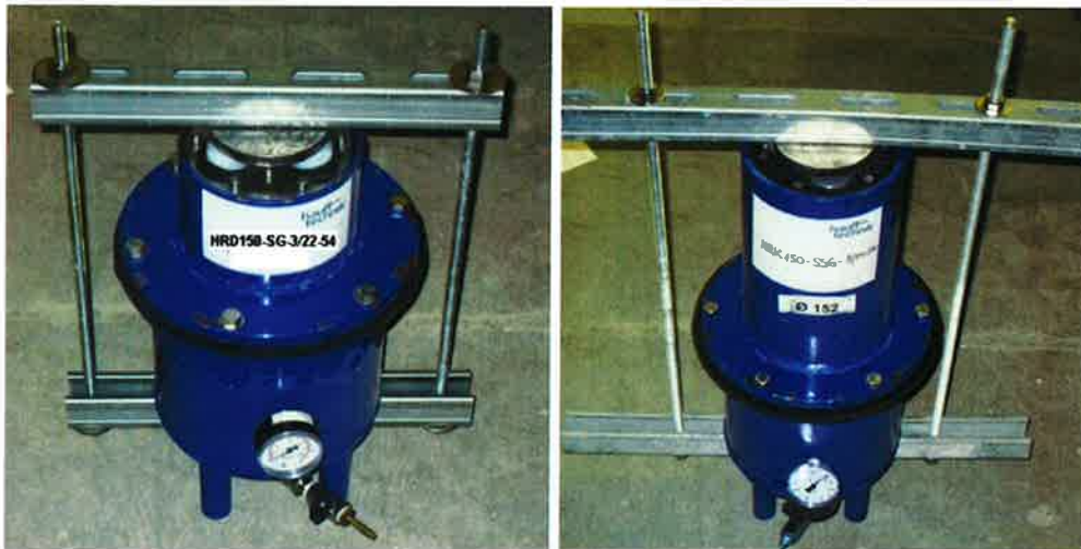
Figure 1. Delivered test setups with already installed press seals HRD150-SG-3/22-54 (left) and HRK150-SSG-3/24-54 (right).
