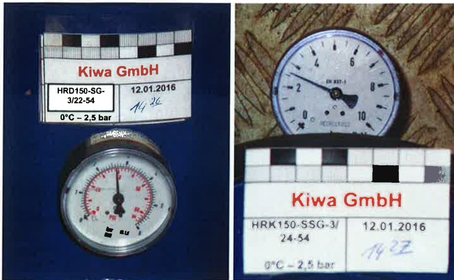
Figure A3. Gas tightness test with the air filled testing cylinder at a nominal pressure of 2,5 bar at 0°C. (Left: manometer display at the beginning of testing with specimen „HRD150-SG-3/22-54“ on 12.01.2016 at 2:26 pm; right: manometer display at the beginning of testing with specimen „HRK150-SSG-3/24-54“ on 12.01.2016 at 2:27 pm).
