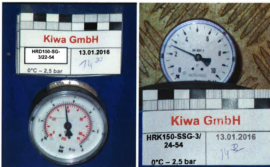
Figure A4. Gas tightness test with the air filled testing cylinder at a nominal pressure of 2,5 bar at 0°C. (Left: manometer display after 24 hours with test specimen „HRD150-SG-3/22-54“ on 13.01.2016 at 2:30 pm; right: manometer display after 24 hours with test specimen „HRK150-SSG-3/24-54“ on 13.01.2016 at 2:32 pm).
