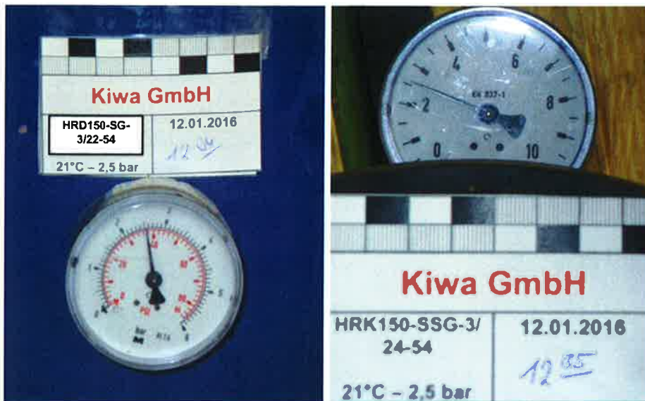
Figure A2. Gas tightness test with the air filled testing cylinder at a nominal pressure of 2,5 bar at 21°C. (Left: manometer display after 24 hours with test specimen „HRD150-SG-3/22-54“ on 12.01.2016 at 12:34 pm; right: manometer display after 24 hours with test specimen „HRK150-SSG-3/24-54“ on 12.01.2016 at 12:35 pm).
