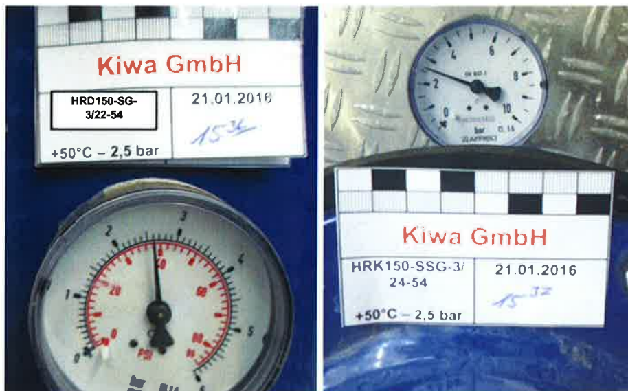
Figure A6. Gas tightness test with the air filled testing cylinder at a nominal pressure of 2,5 bar at 50°C. (Left: manometer display after 24 hours with test specimen „HRD150-SG-3/22-54“ on 21.01.2016 at 3:36 pm; right: manometer display after 24 hours with test specimen „HRK150-SSG-3/24-54“ on 21.01.2016 at 3:37 pm).
