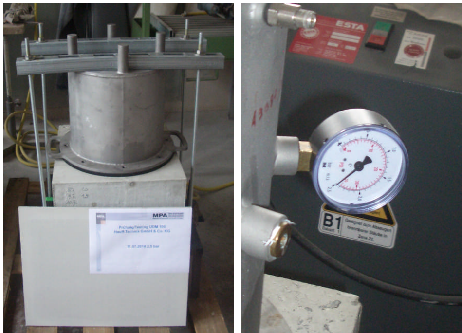
Fig. 3: Condition of the test item after 3 days at pressure step 2,5 bar
