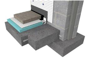
This specification employs 1 form of waterproofing (Type C - Drained Protection) to ensure that the desired internal environment is achieved. The effectiveness of the waterproofing is dependent on the
