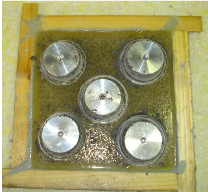
Photo 2-c: After 7 days of polymerization at 20 °C, 5 cylindrical aluminum seals are glued with the epoxy glue PC ® 5800/BL on the with PC ® Leakinject 2K Flex 6811 LV covered substrates in a pattern as described in EN 1542. This photo shows the application of the PC ® Leakinject 2K Flex 6811 LV on the sand blasted metal plate.
