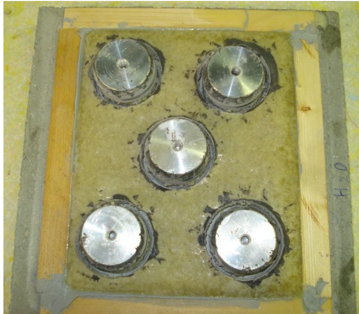
Photo 2-a: After 7 days of polymerization at 20 °C, 5 cylindrical aluminium test dollies are glued with the epoxy glue PC ® 5800/BL on the with PC ® Leakinject 2K Flex 6811 LV covered substrates in a pattern as described in EN 1542. This photo shows the application of the PC ® Leakinject 2K Flex 6811 LV on the concrete slab which was submersed in water.
