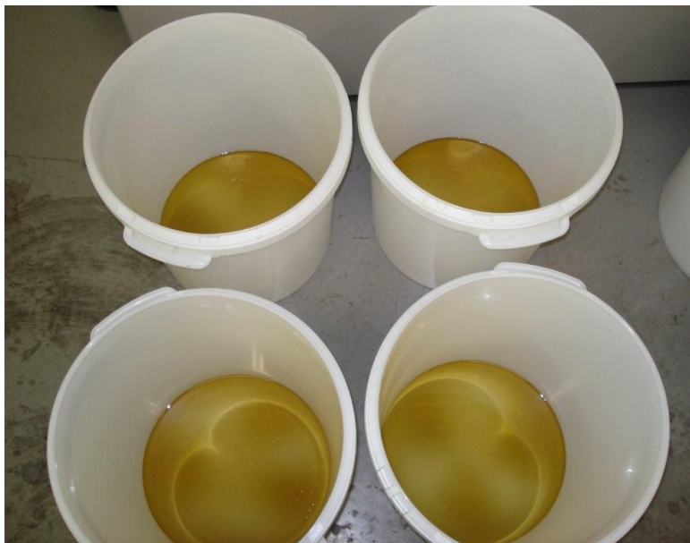
Photo 3: PC ® Leakinject 2K Flex 6811 LV poured into a PE-recipient in a thickness of ± 3 mm.
