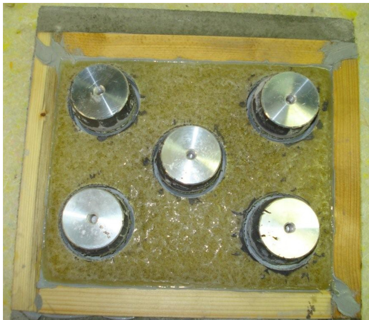
Photo 2-b: After 7 days of polymerization at 20 °C, 5 cylindrical aluminum test dollies are glued with the epoxy glue PC ® 5800/BL on the with PC ® Leakinject 2K Flex 6811 LV covered substrates in a pattern as described in EN 1542. This photo shows the application of the PC ® Leakinject 2K Flex 6811 LV on the dry concrete slab.
