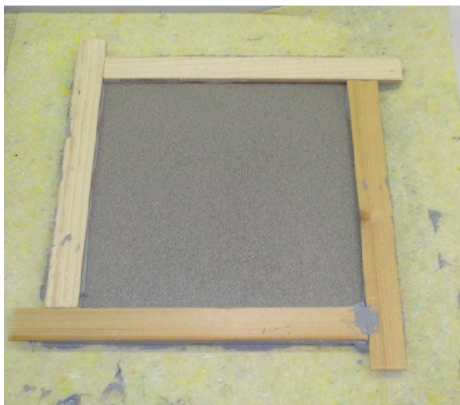
Photo 1-a: A sand blasted metal plate SAE2.5 equipped with a form work.
