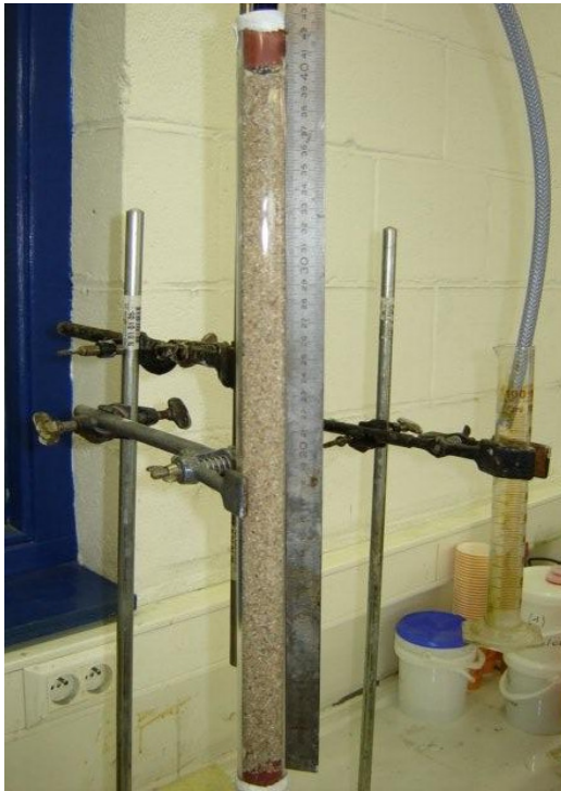
Photo 3 : At the top and at the bottom the injection column is equipped with perforated rubber plugs. Along the sand column, a measuring ruler is positioned.
