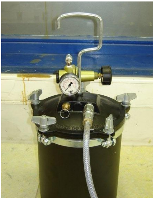
Photo 1 : Pressure vessel that pushes the product through the sand column.
