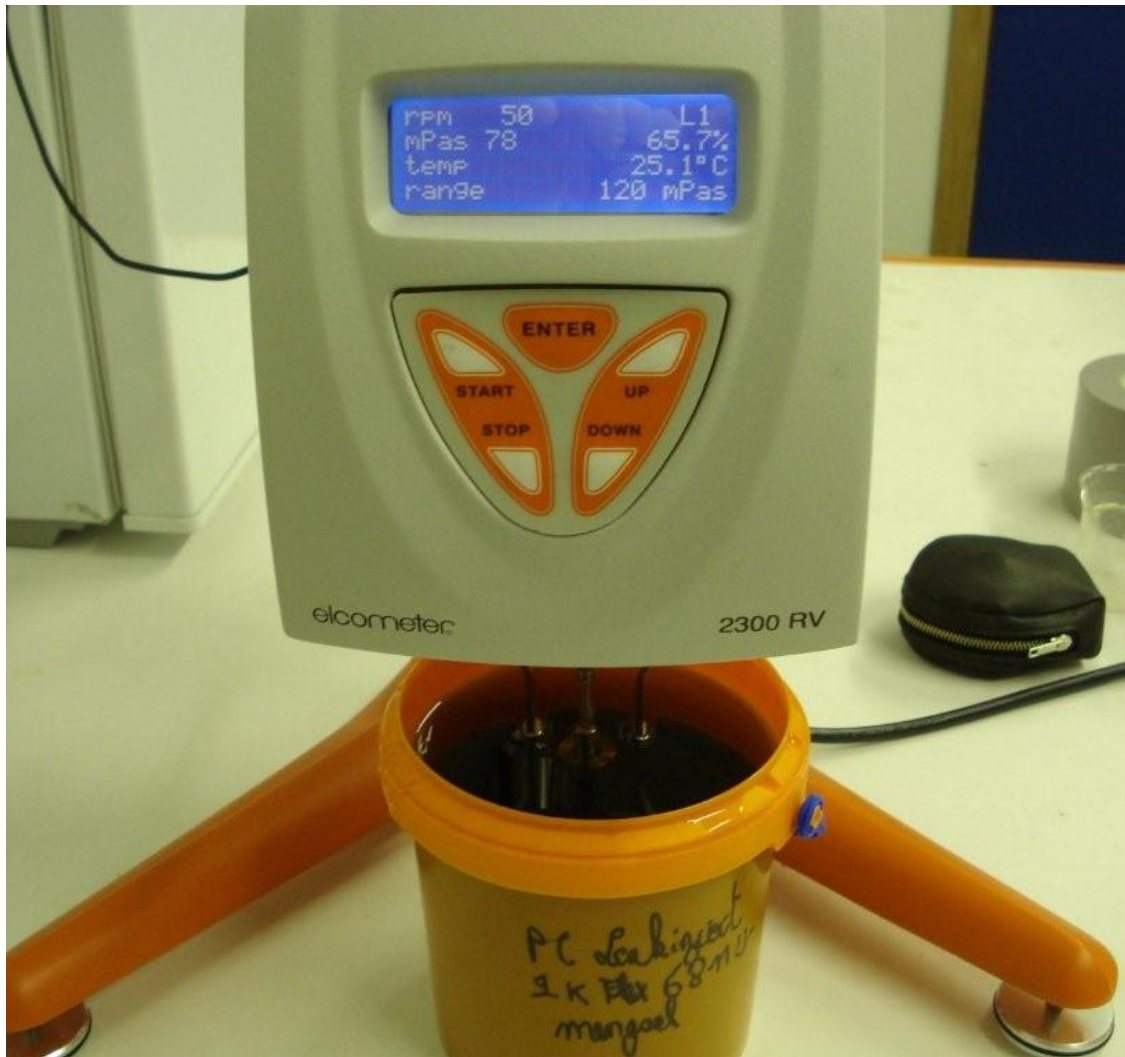
Photo 3: determining the viscosity of PC ® Leakinject 2K Flex 6811 LV.
