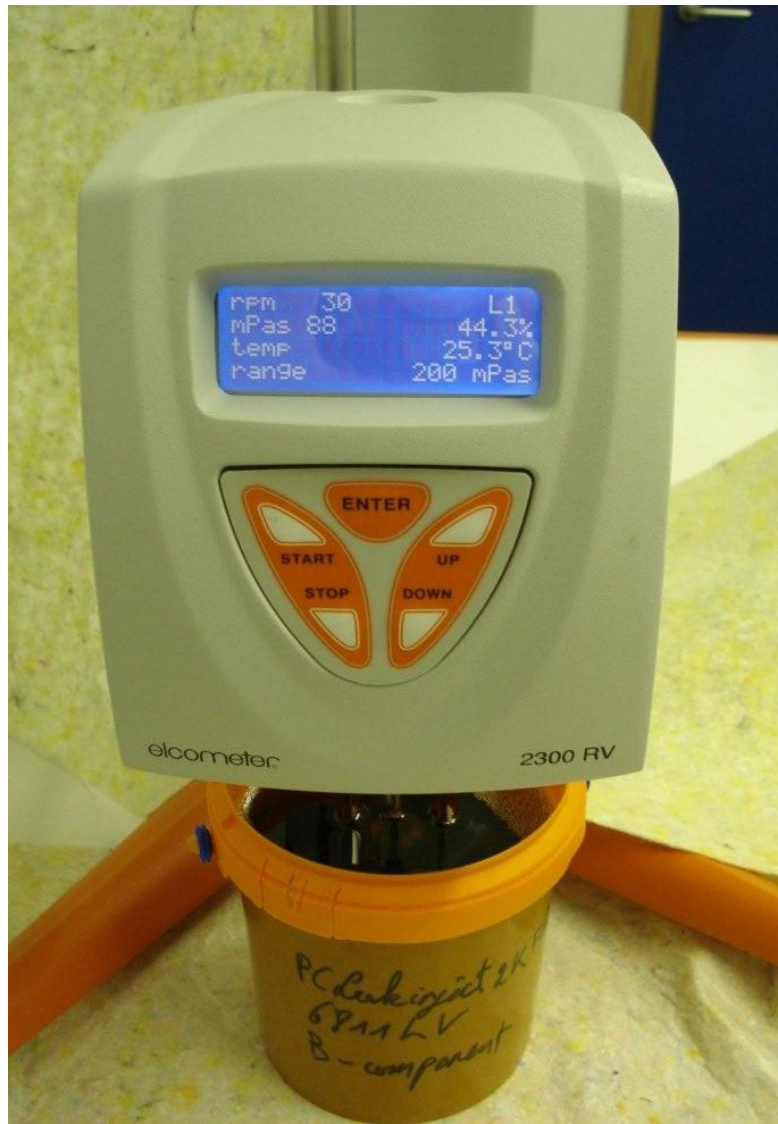
Photo 2: Determining the viscosity of PC ® Leakinject 2K Flex 6811 LV B-component.
