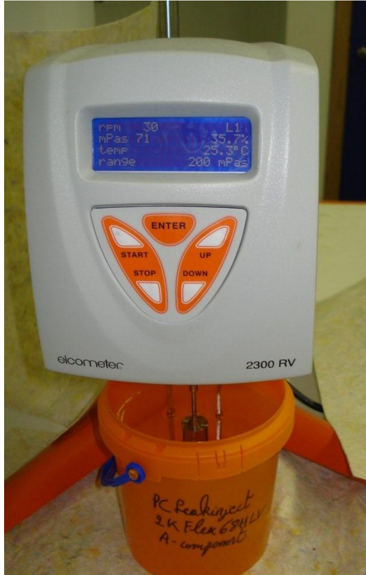
Photo 1: Determining the viscosity of PC ® Leakinject 2K Flex 6811 LV A-component.
