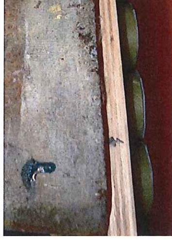
Photo 4: To ensure an intimate contact of the PVC material with the hardened PC® Leakinject 6816/E test pieces, a weight was placed on top of each test specimen.
