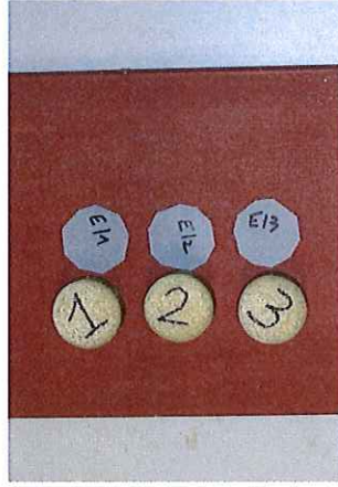
Photo 3: 3 Hardened PC® Leakinject UNI 6816/E samples are placed on top of 3 PVC samples with the same dimensions.
