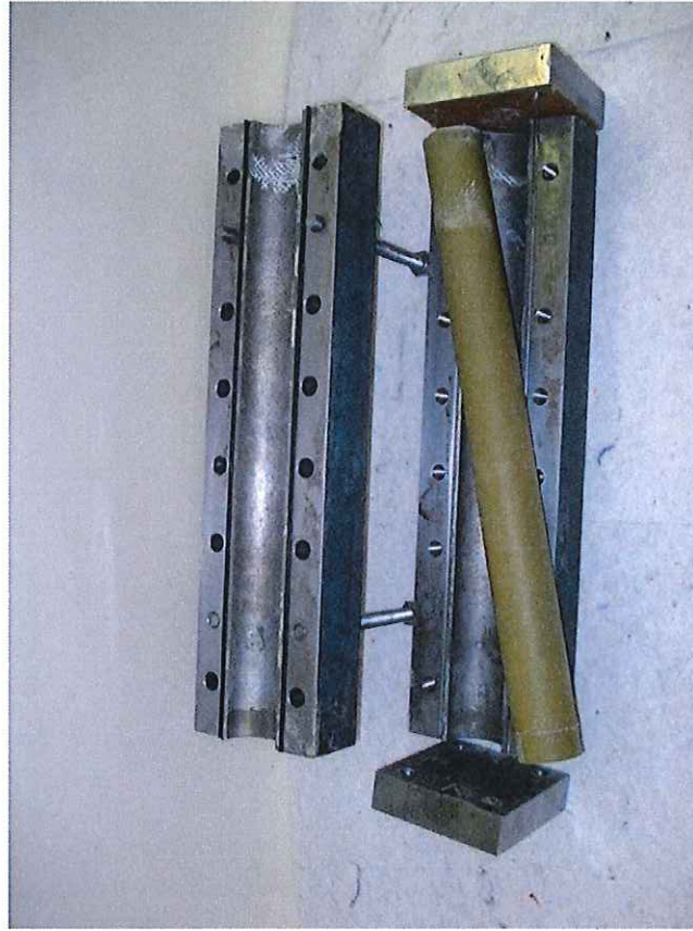
Photo 1: The steel mal in which the PC® Leakinject UNI 6816/E is cured under pressure consists out of 4 pieces.
